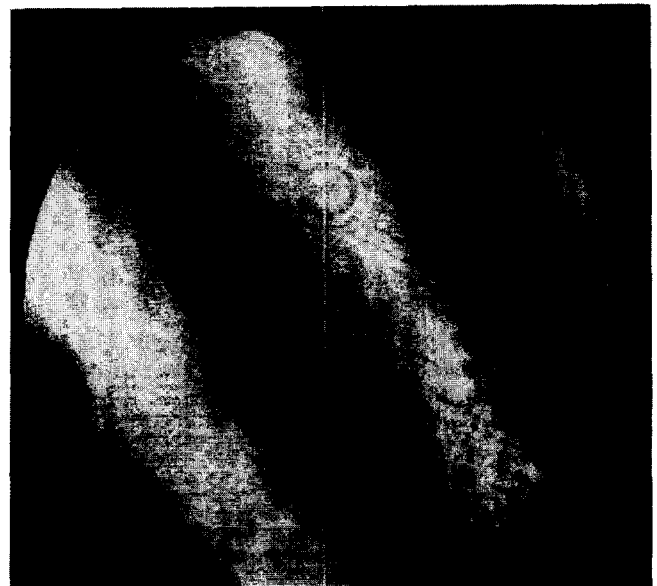
Fig. 13 Ronchigram of a 1.5 kW laser beam
