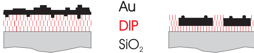
Figure 9.15: Model for the desorption process of the DIP in a system of Au/DIP. On the left side the system is shown prior to the annealing process. The image on the right hand side depicts the situation during and after the annealing step in which some DIP-islands remain unchanged in some regions.
