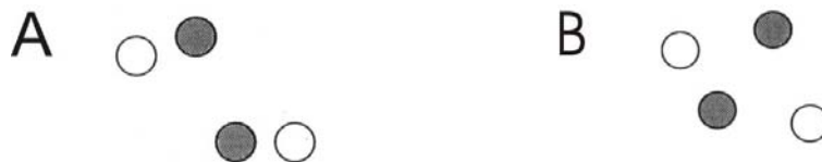
FIGURE 3.12. Temporal assignment of particle coordinates to particle trajectories. The open circles indicate particle positions at time t . One time step later ( t + dt ) the coordinates are represented by filled circles. A) Coordinates can be assigned to trajectories. B) Here, an unique assignment is impossible.
