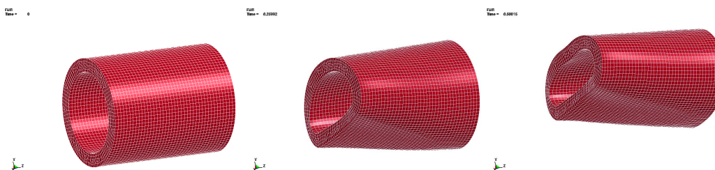
Figure 1.3: Deformation of a steel tube in a drop test, see OLOVSSON AND SIMONSSON (2006).
