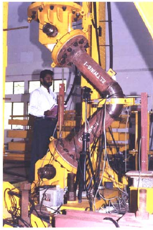
Fig.4.14 Photograph of elbow test set-up
