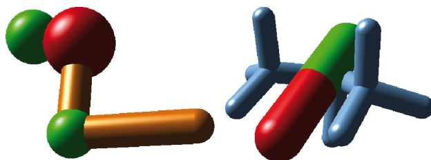
Figure 35: Two complex molecules modelled with spheres and cylinders. Left: an ethanol molecule with the orange stick representing the carbon backbone and three spheres showing point charges; Right: an R227ea molecule with a blue stick representation of the carbon and fluorine atoms and a bar magnet showing a directed charge.
