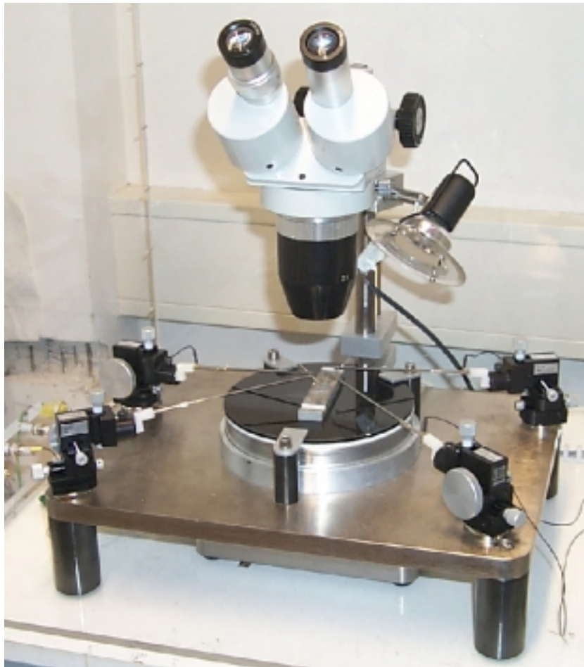
Figure 3.4: Picture of the ex-situ electromigration probe station.
