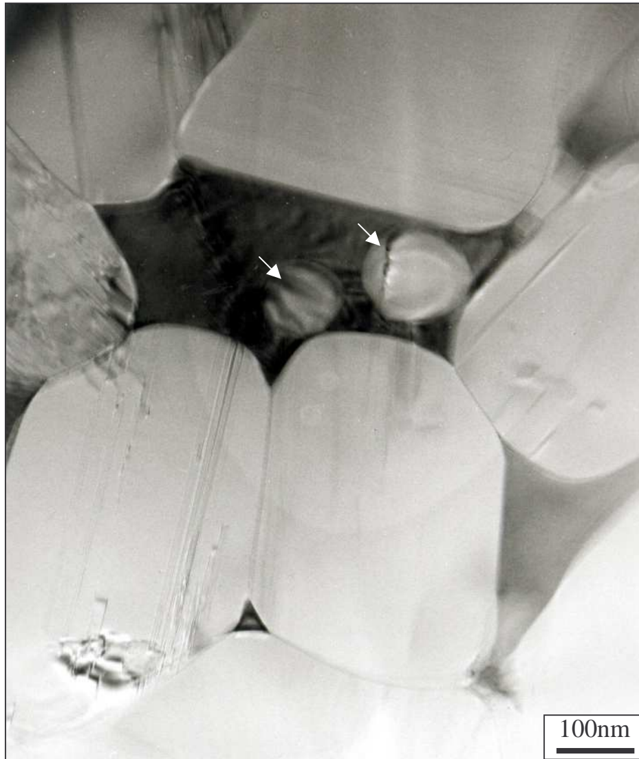
Fig. 6.4 TEM image of 100α-60AlN-Ar, showing typical small SiC grains (indicated by arrows) which have round shapes and are located inside large intergranular pockets, indicating an ongoing solution-precipitation process.
