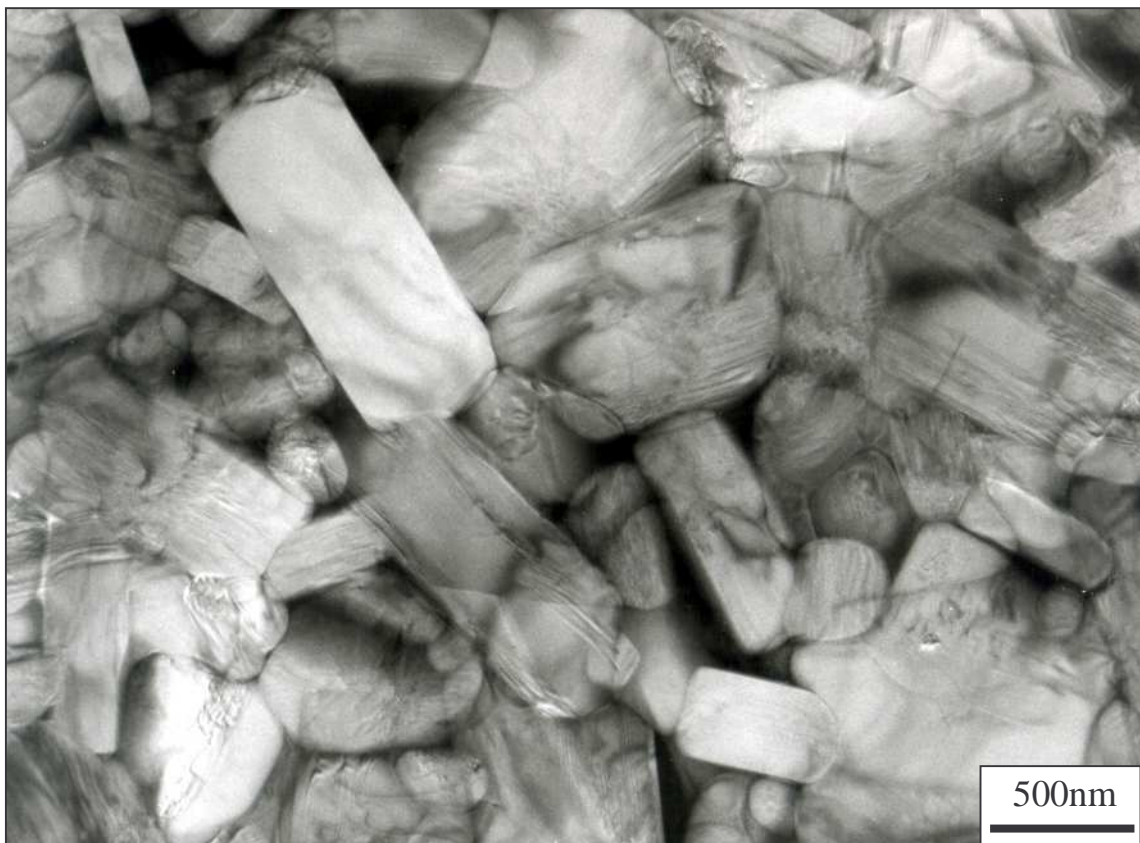
Fig. 6.6 TEM image of liquid-phase sintered sample using \beta -SiC as main component of the starting powder (90 \beta -60AlN-N 2 ). The elongated SiC grains have actually plate-like shape, indicating the \beta -to- \alpha -SiC phase transformation.
