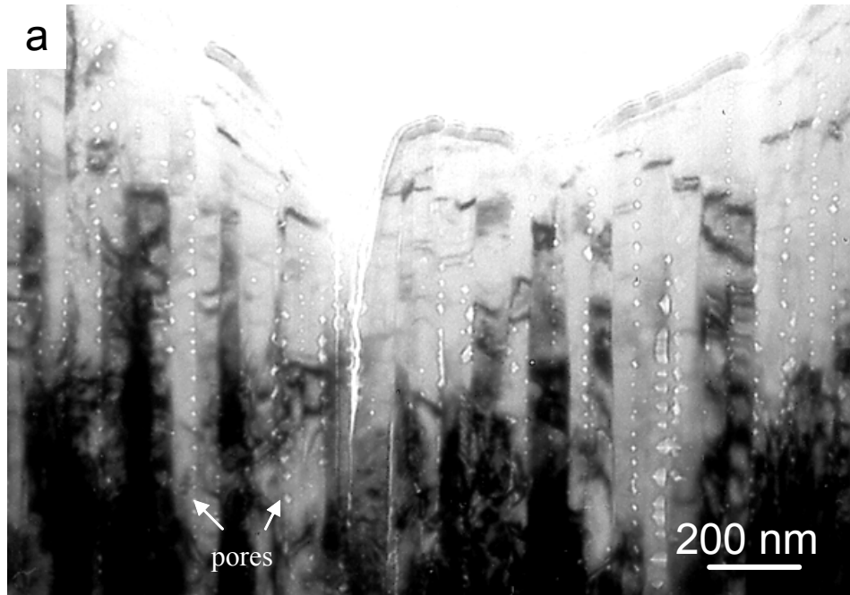
Fig. 5.4 TEM cross sectional micrograph of YSZ coating deposited on a sapphire substrate under stationary conditions: (a) top section ( \sim 1\mu\text{m} above the interface) and (b) bottom section of the columns.
