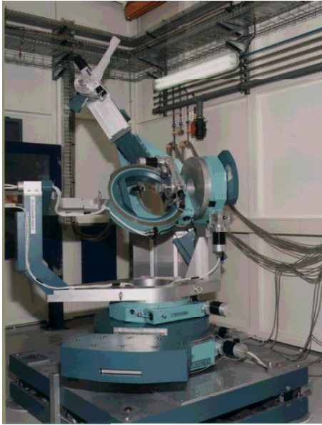
Figure 3.8: Photo of the BM28 diffractometer
