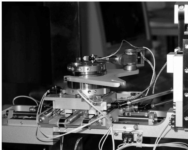
Figure 2.2: Side view of the testing device clamped onto the stage of an SEM Leo 1530 VP (Digital Camera).
