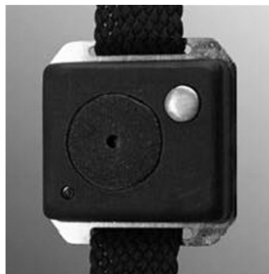
Figure 3.13.: Wrist-Worn Actiwatch Alert Including a Button to Cancel the Alarm (Camebridge Neurotechnology Ltd., 2006)
