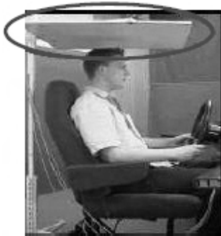
Figure 3.5.: Experimental Setup of the MINDS™ (Whitlock and Pethick, 2002). The Ellipse Indicates the Sensor Position.
