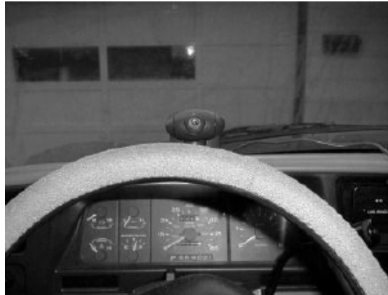
Figure 3.6.: Camera of the Eye Tracking Alertness Monitor System Installed in a Car (Whitlock and Pethick, 2002)
