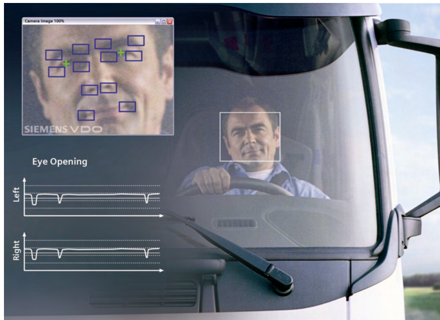
Figure 3.18.: Schematic of the Siemens Driver Attention System (Siemens VDO, 2006)
