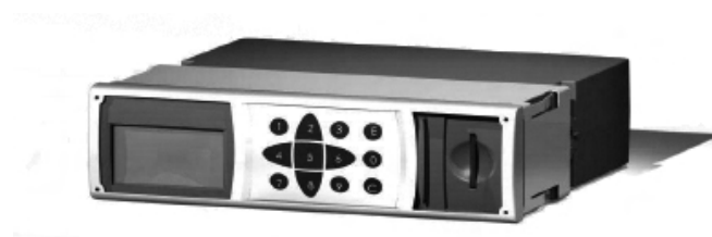
Figure 3.10.: New ASTiD v4.06 Device Sized to Fit into the DIN1 Radio/Cassette Slot in the Dashboard (Pernix, 2006)
