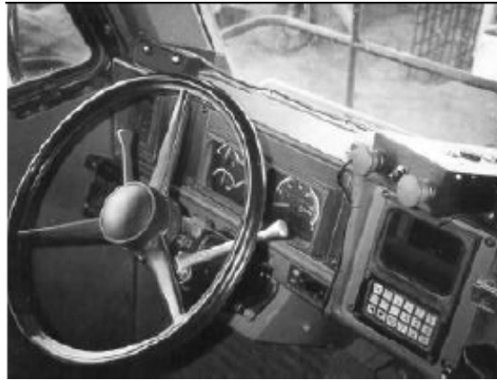
Figure 3.12.: Fatigue Monitoring Device Installed in a Mining Truck. The Stimulus Box is Located on the Left; the Reaction Box is Placed on the Right of the Steering Wheel (ARRB Consulting, 2006)
