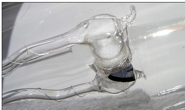
Figure 5.13: The OSC No. 3 sample before the first electrocatalytic experiment in the SC reactor. The Pt-net electrodes were well-separated and made no short circuit.
