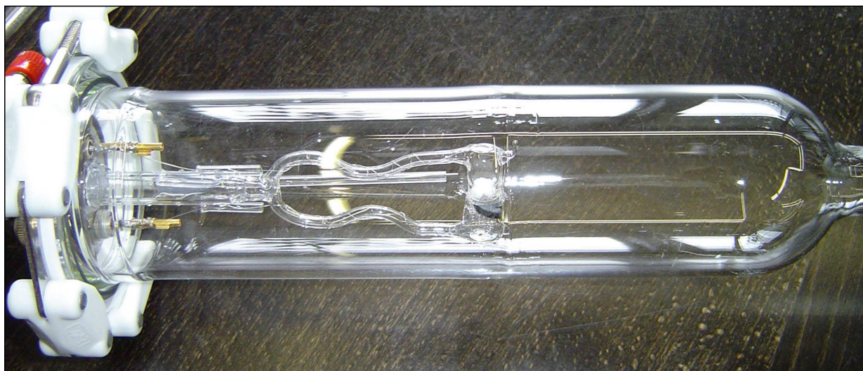
Figure 5.7: (a) The quartz ‘fork’ is the sample holder used for a single chamber reactor, which can supply a single gas mixture at both sides of the sample. (b) The single chamber reactor which serves simultaneously as IS-measurement and electrolysis cell. All glass parts are made of quartz. An \text{Li}_3\text{N} sample, sandwiched with two platinum nets electrodes, is mounted between the two quartz branches which can supply a single gas composition. In operation, the gases were supplied from the left-hand side and were leaving the reactor through an outlet (not seen completely in the photograph) to the FTIR.
