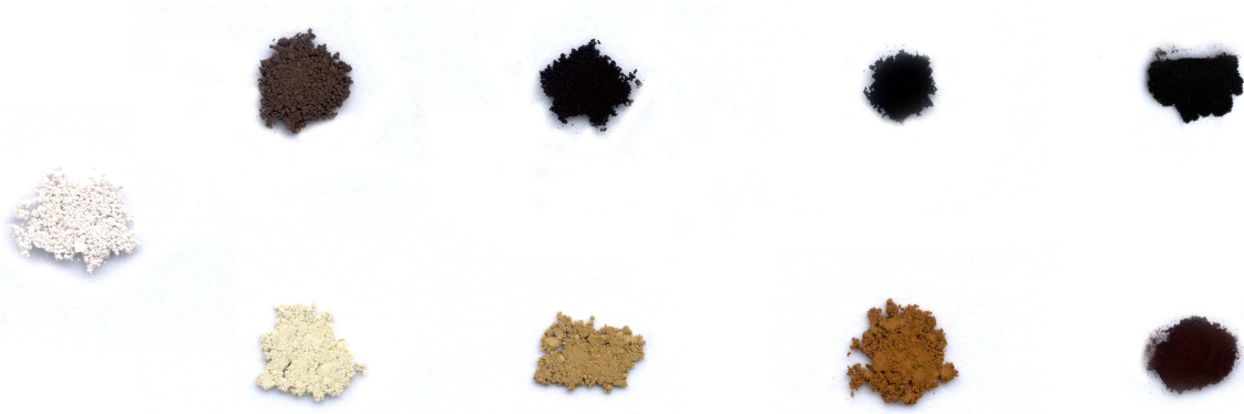
Figure 2.5: Sample photographs. The leftmost sample is the undoped \text{SrTiO}_3 ; upper row: oxidized samples, lower row: reduced samples. In both rows iron content increases from left to right: x = 0.01 , 0.1, 0.3 and 1.
