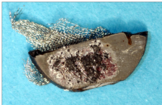
Figure 5.16: Observed lithium-ion mass transport in the OSC No. 3: (a) the anode side, the electrode imprint clearly shows that electrolysis occurred; (b) the cathode side, where the newly formed material can be seen.
