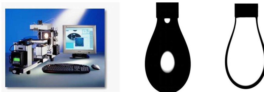
Figure 4.6: The instrument OCA 30 used for the pendant drop measurements (left). A picture of a pendant drop of pure water surrounded by air (center) and picture of a pendant drop of [\text{hmim}^+][\text{Tf}_2\text{N}^-] immersed in n-hexane (right) as recorded with the OCA 30.
