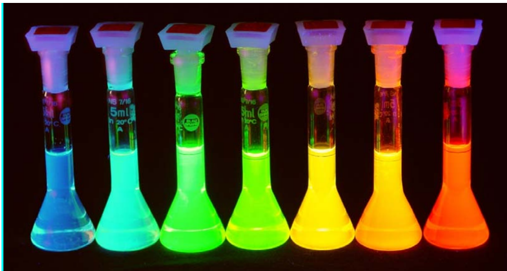
Fig. 1.7. Fluorescence of colloidal CdTe nanoparticles of different size (reprinted with permission) [47].
