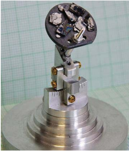
Figure 3.7: Photo of a mosaic of co-aligned Mn-doped BFCA samples. The orientation of each sample was checked by X-ray Laue diffraction.
