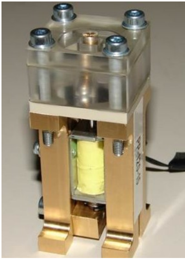
Fig. 22 Valve demonstrator with a flexible mounted seal seat
