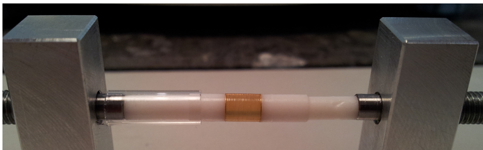
Figure 5.5: A formed membrane stack with gold electrodes on both ends. The vise compresses the stack to ensure cohesion.
