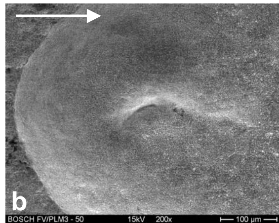
Fig. 3.6: Scanning electron micrographs: (a) trough formations on the 100Cr6 surface, (b) single trough on the 100Cr6 surface, and (c) centre of the trough shown in (b): carbide segregation.
