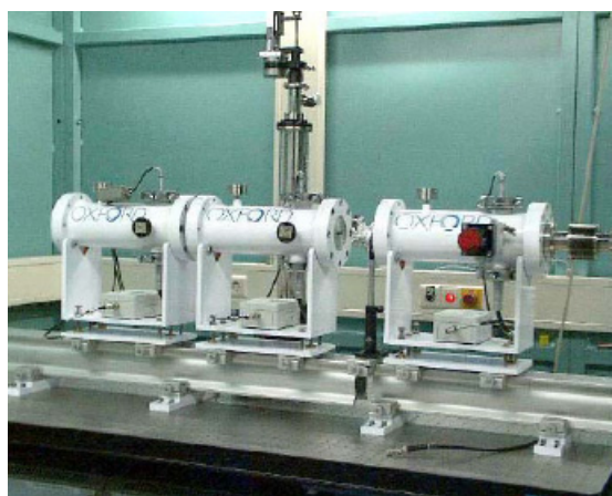
Figure 3.1.3. Picture of ionisation chamber. [Photograph from the XAS beamline at ANKA, Karlsruhe].
