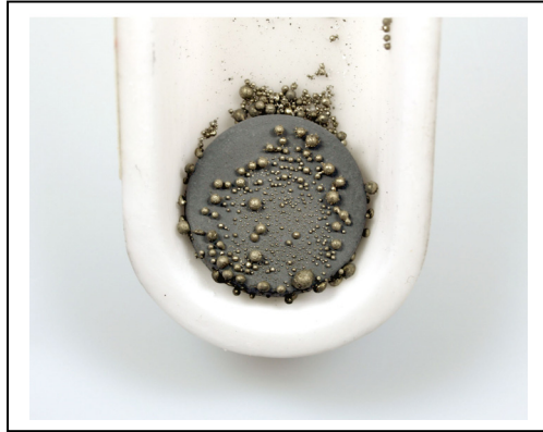
Figure 4.1 Nickel cermet after exposure to H 2 + H 2 S (1 vol%) at 750°C for 3 h.
