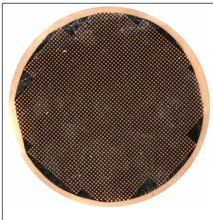
Figure 3.1 Ni patterns made by photolithography (the small squares are the surface of the electrolyte where there is no Ni and their size is 70\ \mu\text{m} \times 70\ \mu\text{m} )
