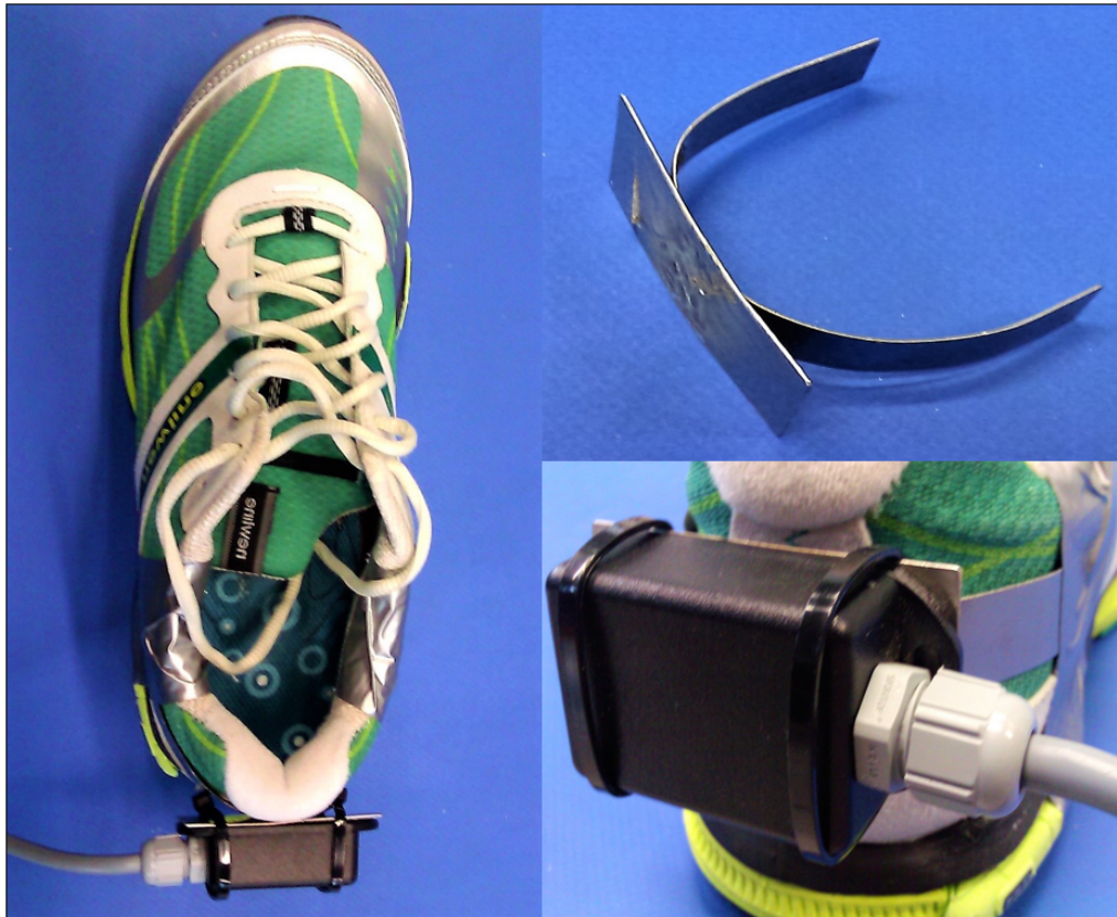
Figure 11: The IMU was affixed to a metal clamp and mounted onto the shoe's heel cap to allow recordings during running.
