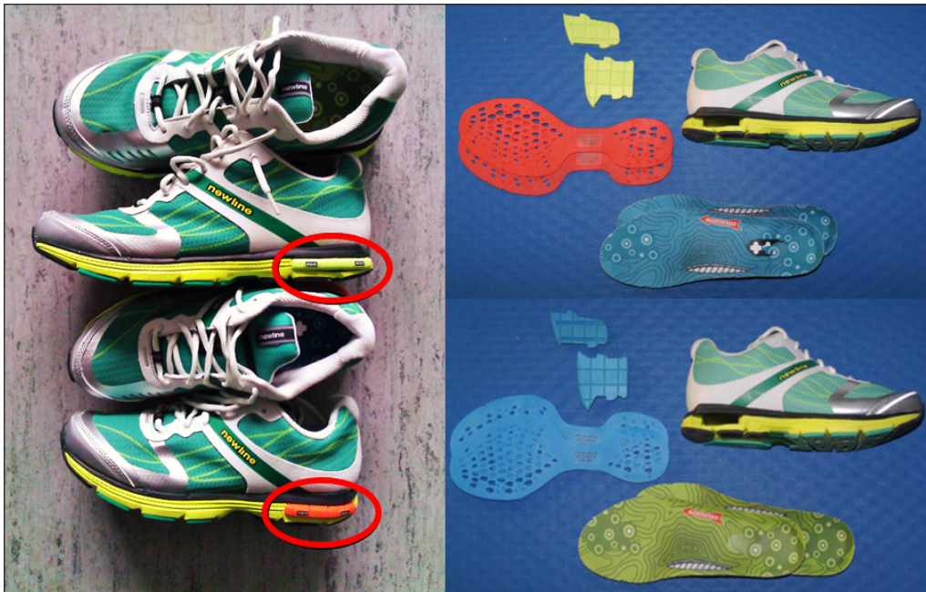
Figure 13: The modular running shoe was used to set up two different configurations of this shoe. Damping material and insoles can be exchanged in this shoe to obtain individual configurations.
