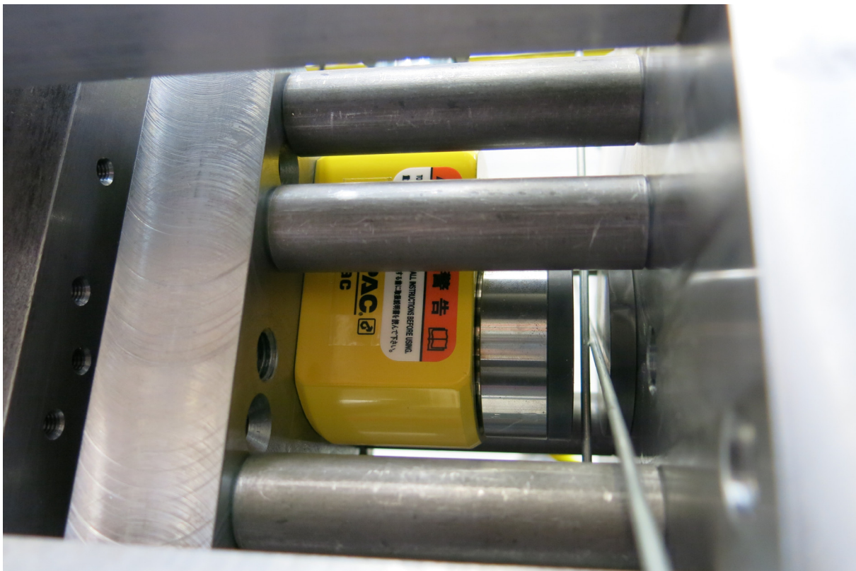
Figure 3: Detail of device to press two wires against each other
