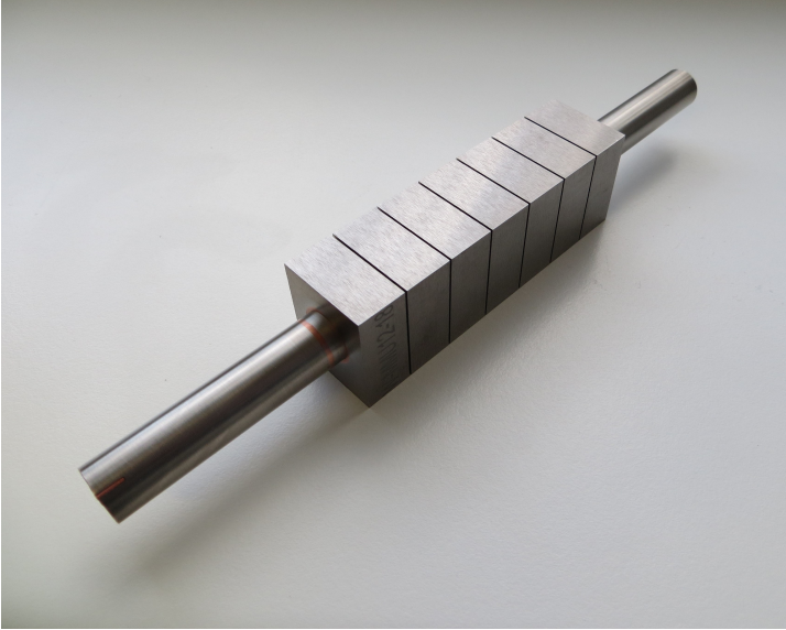
Figure 5.1: An as-received mock-up, produced by Plansee SE , that consists out of 7 tungsten monoblocks which are joined to a CuCrZr cooling tube. This mock-up is identical to the W-MMU-12-16 mock-up used in the experiments.
