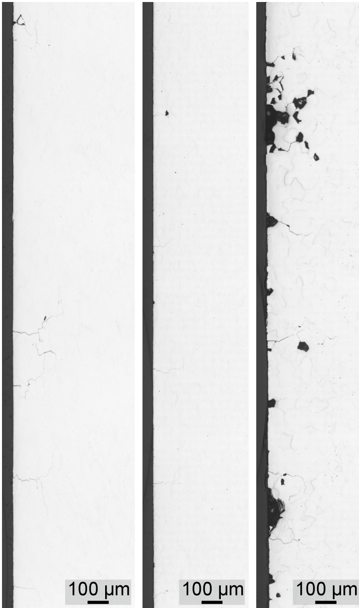
Figure 4.4: LM pictures of a polished cross section of the cracked samples, which were exposed in JUDITH 1 to HRT-12 after a pre-exposure in GLADIS with S-H (left), M-H (middle), and L-H (right). For the L-H pre-exposed sample a substantial amount of grain loss, that occurred during sample preparation, is visible.
