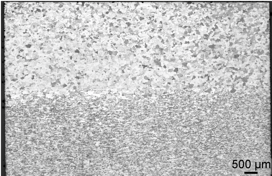
Figure 4.12: LM pictures of an etched cross section of a sample loaded in JUDITH 1 to H400-12 after pre-exposure in GLADIS with L-H/He. The area of recrystallization and grain growth, 3.5 mm to 4 mm deep, is distinguishable from the bulk material.
