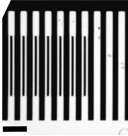
Figure 4.21.: Modified geometry of the microcantilevers is shown (left side). In this way, center of these microcantilevers is etched through. In comparison to the ordinary geometry (right side), they can yield in larger ZPF and consequently larger spin-phonon coupling parameter. Scale bar shows 20 \mu\text{m} .
