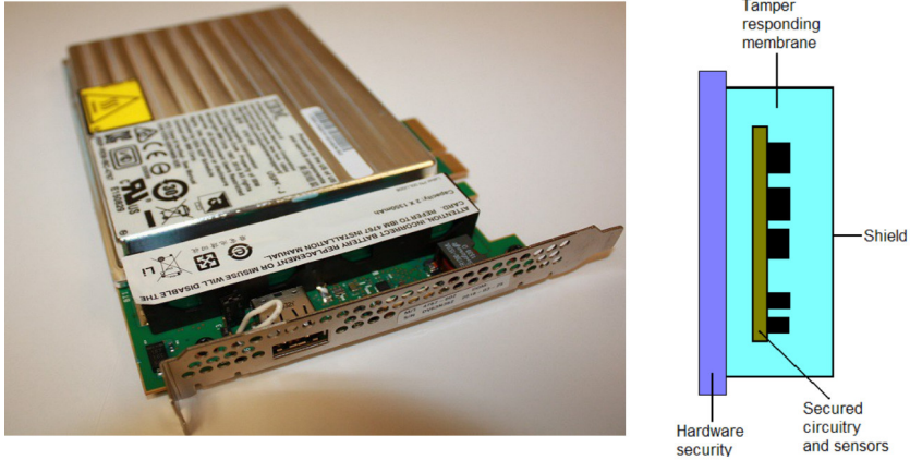
Figure 2.3: IBM 4767 PCIe HSM with secure enclosure [IBM].
