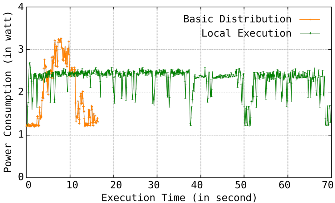
Figure 4.15.: Power consumption on the smart phone for a local execution and the basic distribution of the mobile application.
