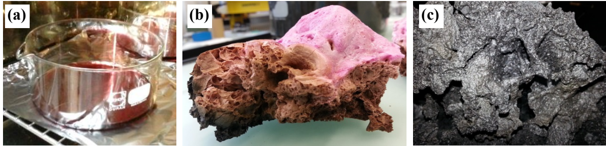
Figure 4.1: Steps during soft chemistry synthesis: (a) Clear pink solution containing the complexed metal cations. (b) Partly dried xerogel recorded during the drying process. (c) Xerogel after drying.
