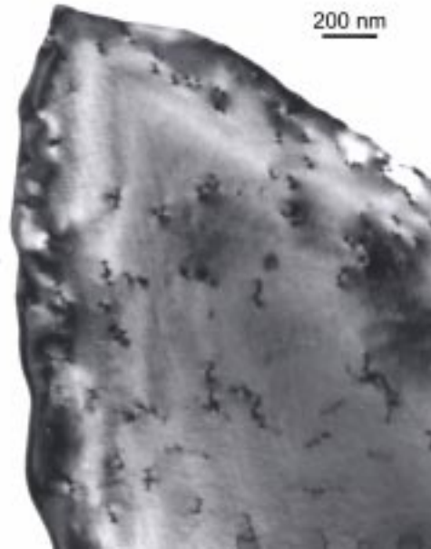
Figure 4.4.: Bright field TEM image of the homogeneous solid solution of Pd 94 B 6 after annealing of the bulk material at 628 K for 70 days (=demixing, cf. Fig. 4.5) and subsequent annealing at 973 K for 1 hour. Hereby a homogeneous solid solution is established.
