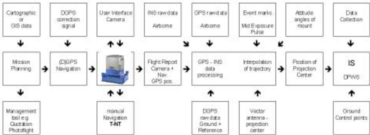
Figure 7 : Dataflow at the beginning of the digital process-chain
