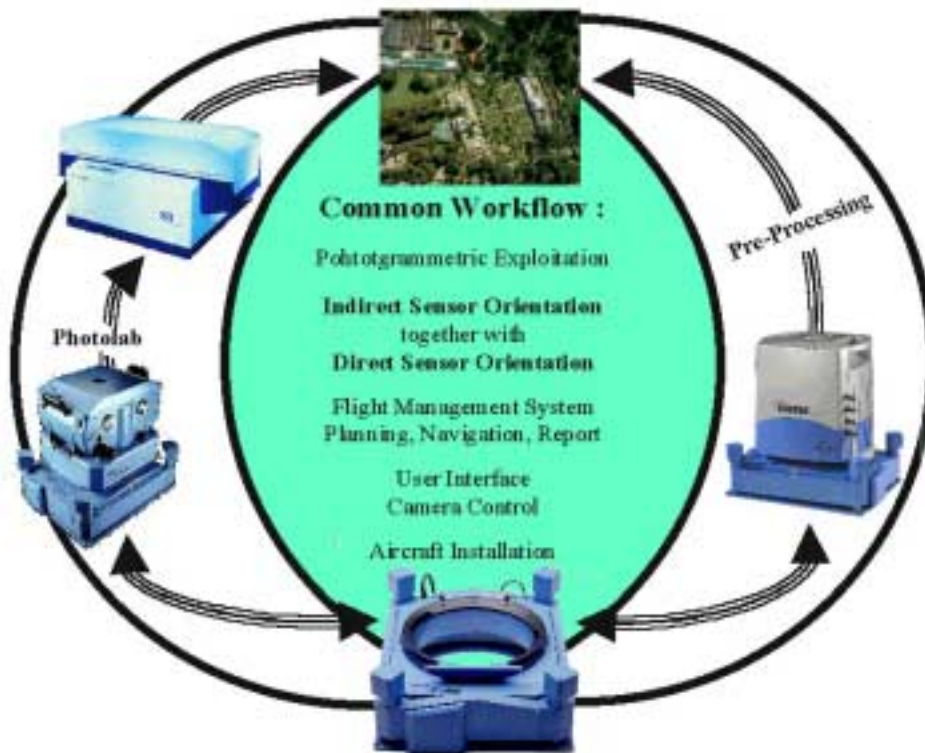
Figure 6 : Complementary use of digital and film-based camera within the same installation
