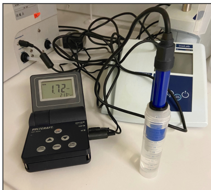
Figure 7.1: Picture of the O 2 -meter used for the preliminary experiments. One can see the device on the left-hand side of the picture, displaying the DO content measured by the electrode inserted in the tube containing the water sample.
