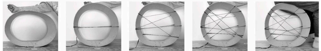
Figure 5. Initial study sequentially placing carbon FRP on a thin timber element, reinforcing most deformed regions.
