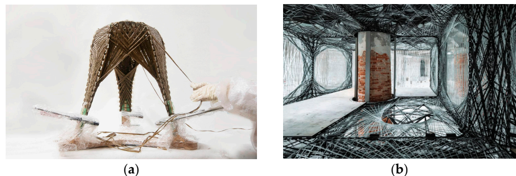
Figure 2. State of the art: (a) FlexFlax stool embedded winding frame [13]; (b) hybrid timber-fibre slab of the Maison Fibre [11].
