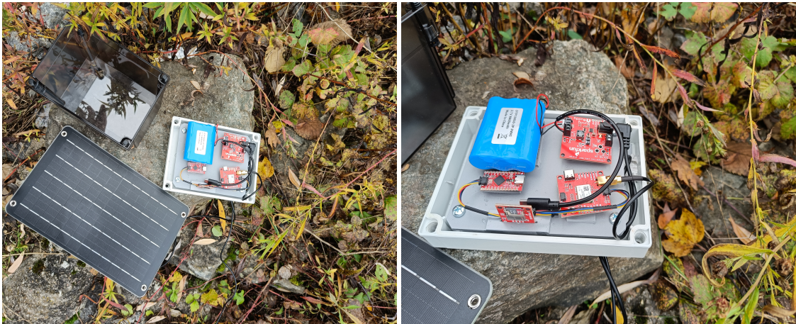
Figure A.1.: SparkFun self-constructed GNSS receiver
