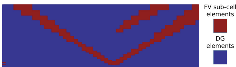
FIGURE 11 Distribution of the DG and FV subcell elements in the oblique SWLBLI flow field [Colour figure can be viewed at wileyonlinelibrary.com ]
