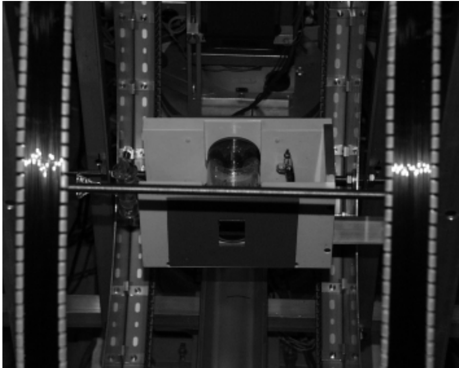
Figure 9.4: Photograph of the ^3\text{He} spin filter cell, placed inside the Braunbeck coils and masked with \text{B}_4\text{C} .
