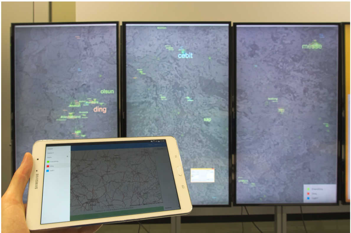
Figure 4.2: Photo of our tablet application in use. Most of the area is occupied by the map. The slide-out menu on the left provides a list of layers. On the right, text filters for the current layer are edited. The bar at the bottom allows filtering by time.
