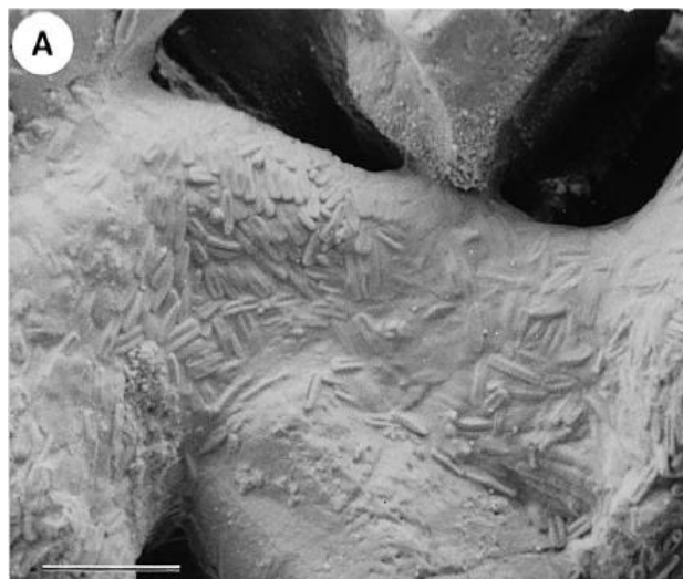
Figure 2: ESEM image of a natural biofilm in an intertidal mudflat habitat (de Winder et al., 1999): the thick layer of EPS produced by the biofilm consisting of different diatoms has glued the sediment grains together so that no individual grains remain visible; scale bar: 250 \mu\text{m} .
