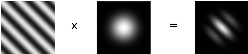
Figure 3.11 — A sinusoidal function is multiplied with a Gaussian function to generate a Gabor filter.
