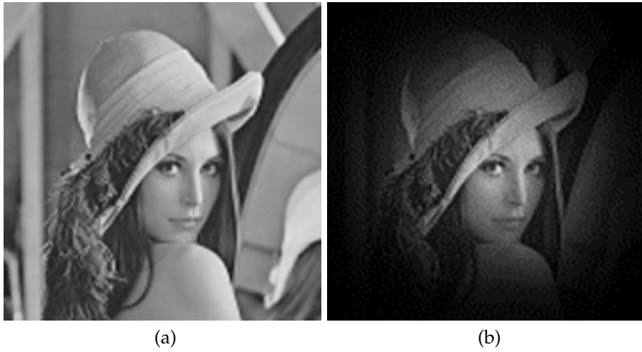
Figure 3.4 — (a) shows the input image, and (b) after applying the Hamming window.
