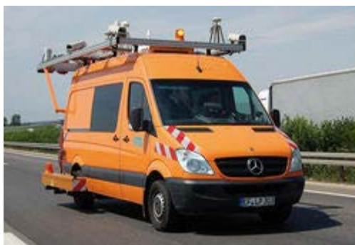
Figure 6.1: S.T.I.E.R. mobile mapping system (LEHMANN+PARTNER 2014).
