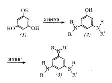
The reactions are carried out with an excess of amine (phloroglucinol : amine = 1:4), the molar ratio (2):(3) obtained depending solely on the reaction temperature. The products can be purified by fractional distillation or recrystallization.
