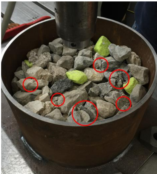
a: breakage on the surface
