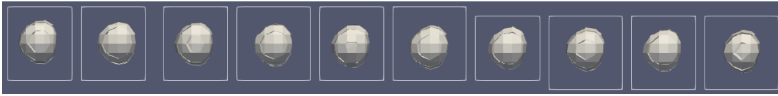
Figure 5.9: Rendering of the example droplet with low error over time. The surface was reconstructed using PLIC. Only a part of the trace for this droplet is shown.
