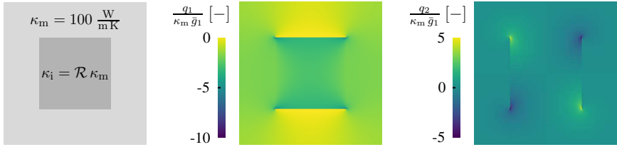
Figure 6.5: Left: unit cell with one square inclusion (25% volume fraction). Middle, right: components of the heat flux field computed with FP-FANS for \mathcal{R} = 100 and for the resolution 2048 \times 2048 .
