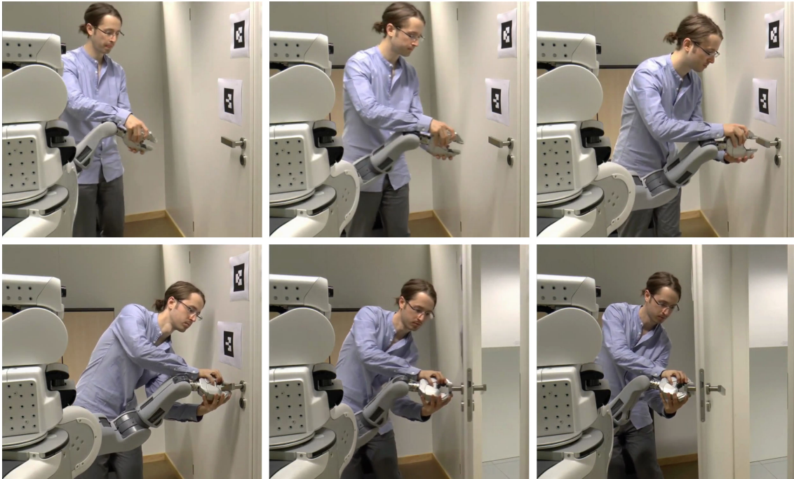
Figure 8.8: Door experiment (see Section 8.1.5) — Demonstration of a skill via kinesthetic teaching.
