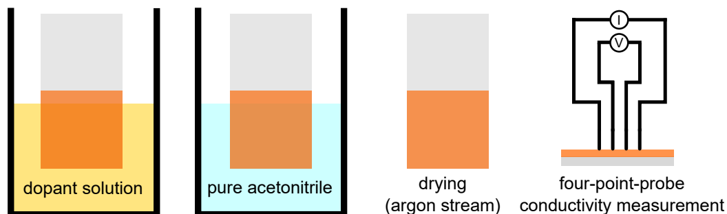
Figure 5.32: Sequential method used for chemical doping of thin films of PT-TPA and PT-spTPA , followed by conductivity measurements.
