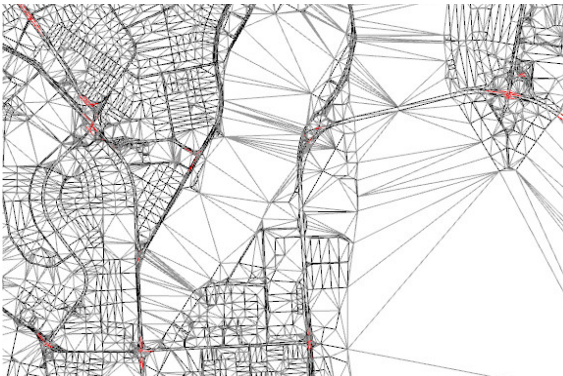
Figure 3.1: Spherical Delaunay triangulation (gray) constrained to contain all line segments (black) of streets in Ecuador. Intersections of constraints are given in red.
