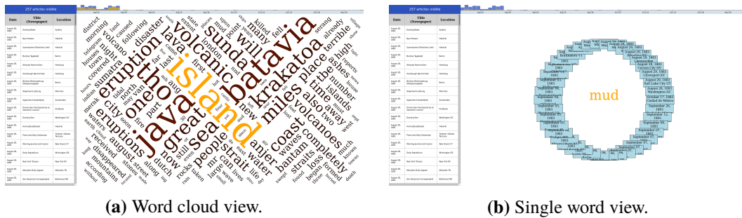
Figure 4.5: Implementation version v0.7 . In the word cloud view (a) a word cloud of the most used words in all documents (sans stop words) is shown. On hovering over a word, it and the data it represents is brushed in the word cloud and the date histogram. Clicking on a word switches to the single word view (b), where the word is shown in the centre and the document nodes containing the word are drawn around it.
