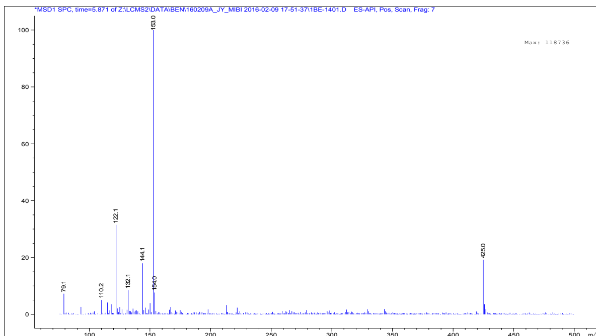
Appendix-A3. ESI mass spectrum of 4-APA standard. Recorded by Agilent 6130 mass spectrometer, TOF-Q system in the positive field of view. The strongest signal corresponds to the mass of the H^+ adduct to 4-APA ( m/z = 153 ).
