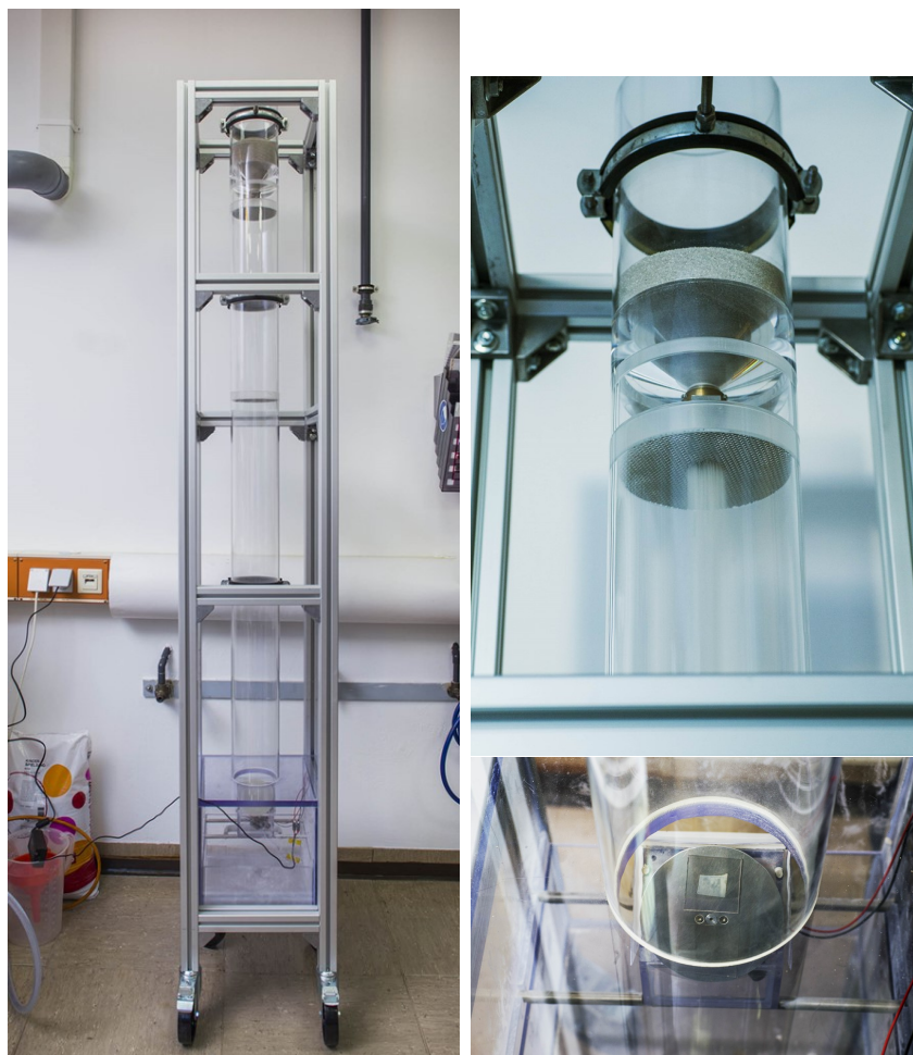
Figure 4.5.: Images of the sand trickling test stand corresponding to the standard DIN 52348.
