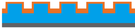
Figure 1.1.: Schematic drawing of a superhydrophobic PU film created by hot embossing of microstructures and subsequent plasma enhanced chemical vapor deposition (PECVD).
