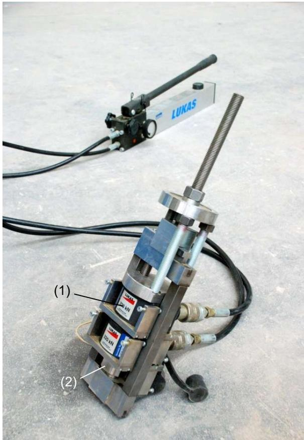
(1) Hydraulikzylinder, (2) Kraftmessdose
